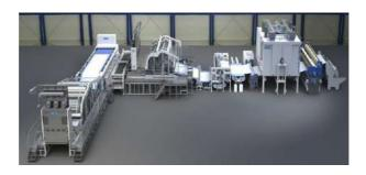
Spunlace - is a nonwoven fabric that uses fibers, the most popular of which are viscose and polyester staple fibers. Spunlace nonwoven fabric is a product of the process of entangling a web of loose fibres through multiple rows of jets of water at high pressure which pierce the material and tangle the fibres.
