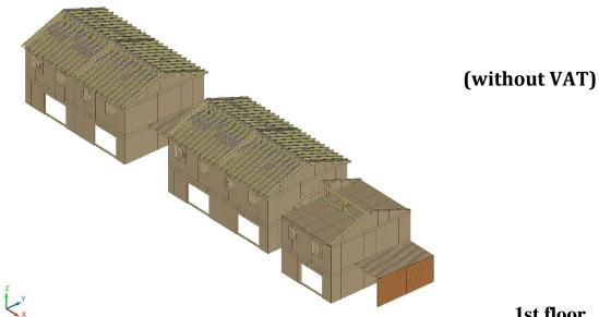
**Homekit:**set of panels panels for walls, overlaps frontons, additional elements (truss system, heat-insulating slab of slagwool, OSB, waterpro of the roof and walls, vapor barrier film, gypsun set of metalware for the assembly of wall panels, partitions.
